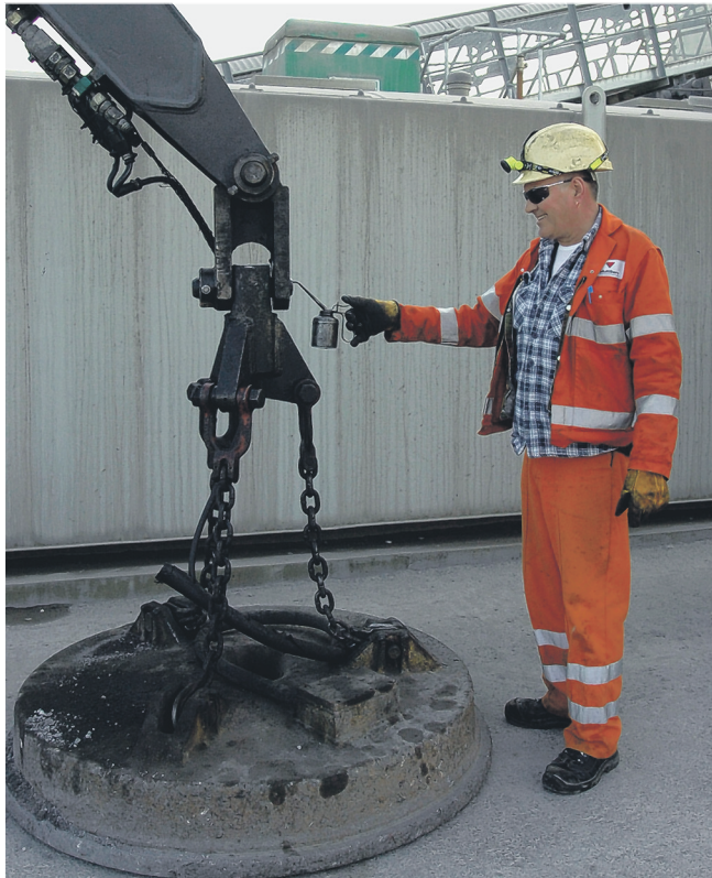
Heavy machine: Stuart Rodgers oiling links on the electro magnet
