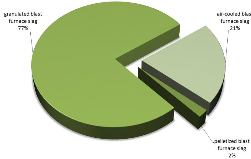
Use of **blast furnace slag**: 32.2 million tonnes
