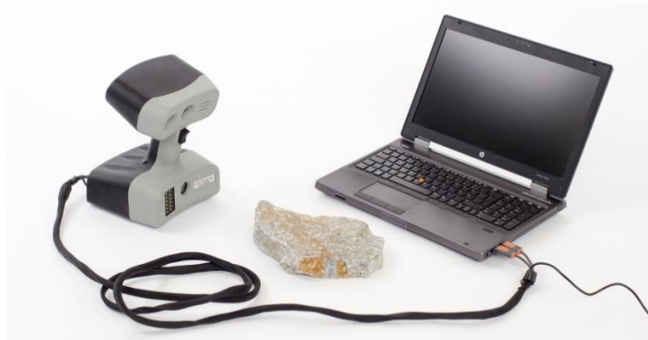
Figure 4: Measuring by a hand-held scanner
