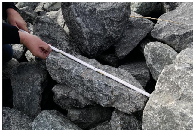
Figure 2: Stone with a length to length-to-thickness ratio greater 3
