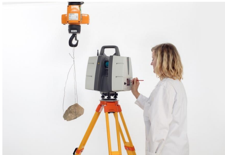
Figure 5: Measuring by laser scanner
