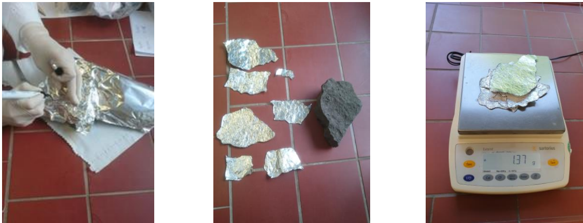
Figure 3: Aluminium foil method for surface determination, tear down of foil pieces
